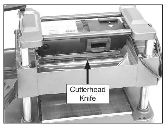
**Figure 28.** Location of cutterhead knives and cap screws.
